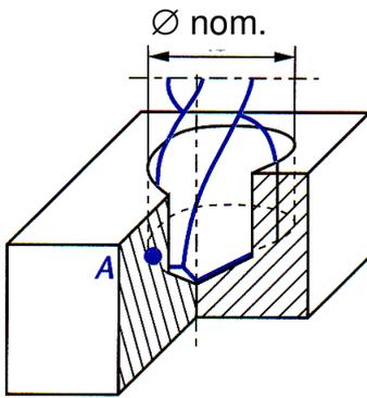
$$\text{Ø perçage} = \text{Ø nominal} - \text{pas}$$
